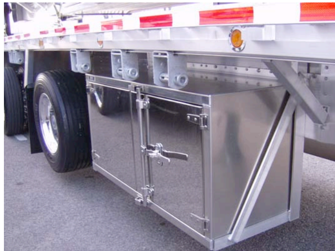
--Example of Support Brackets --
